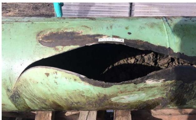
*Photo:* A fatigue crack was the **probable cause** of a 2017 pipeline rupture in South Dakota that spilled thousands of gallons of **crude oil**, according to a **pipeline accident brief** released by the **National Transportation Safety Board** (NTSB).
