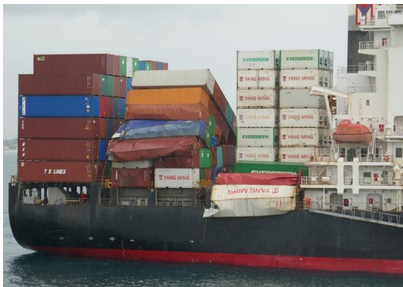
Photo: Collapsed containers are seen on the deck of the YM Efficiency upon its arrival at the Port of Botany on June 6, 2018. Photo: ATSB
