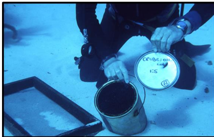
Photo 2. Pre-mixed crude oil & sinking agent with screened frame.
