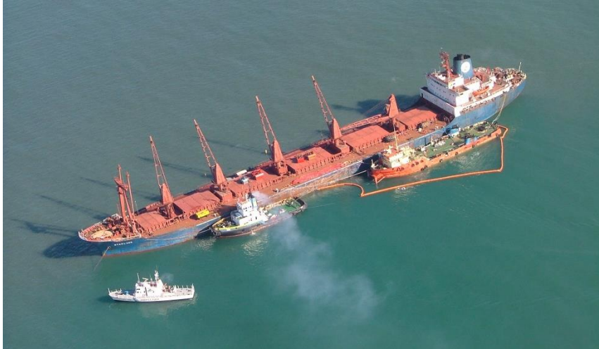
Above: Bunkers lightering of grounded vessel, Necochea, Argentina.
