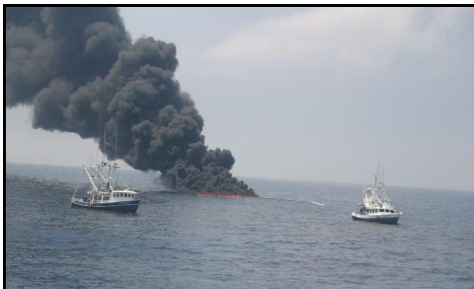
Photo #3 - Towed Fire Boom Configuration with Ongoing Burn of Crude Oil
