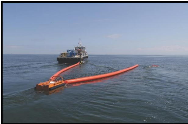
Photo #1 – Large vessel with towed recovery system
