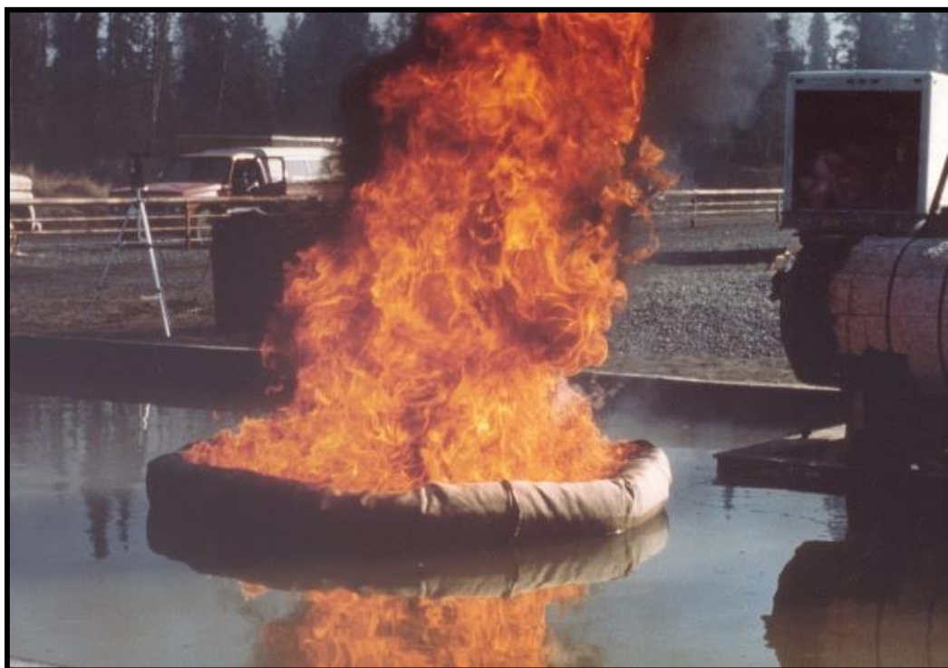
Photo 1. Experimental fire boom test in Kenai, Alaska, 1983.
