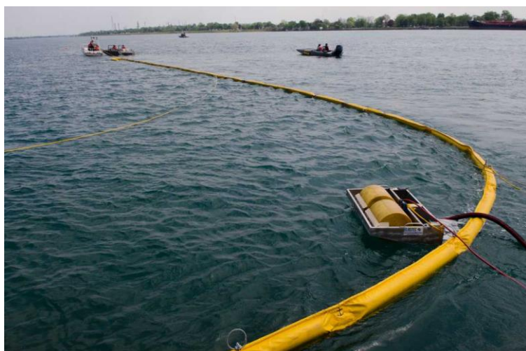
Photo: A skimmer floats in the trapped area and would suck up spilled material as small boats pull the large yellow boom during a 2016 oil spill exercise by U.S. Coast Guard and local agencies. MARK R. RUMMEL, TIMES HERALD
