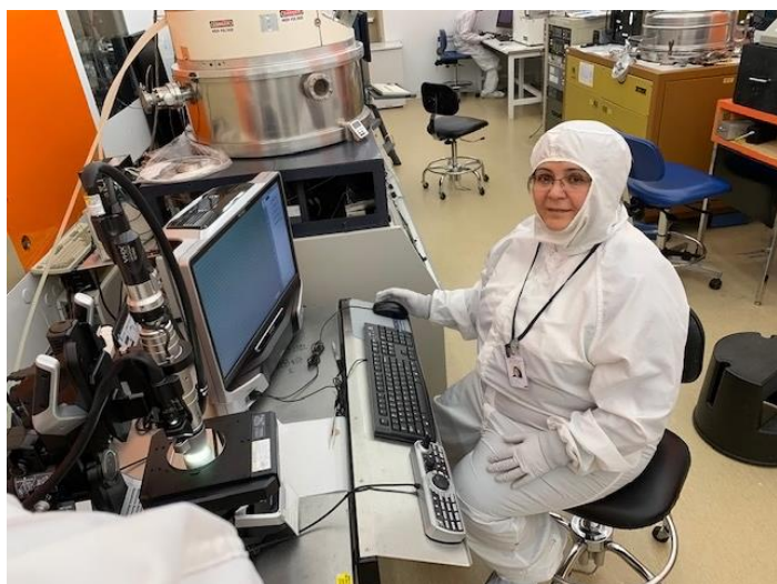
Photo: The monitor screen, which is connected to the microscope computer, shows oil droplets. The printing process is done in a cleanroom environment to control temperature, humidity, and air particle count. The cleanroom smock (white outfit) is made of a fabric which does not shed particles and fiber. Photo credit: Terry Brough at the Minnesota Nano Center.
