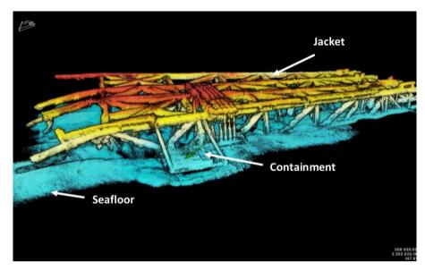
Picture - An echoscope image showing the toppled platform with no plumes coming from the seafloor following the installation of the containment system.
