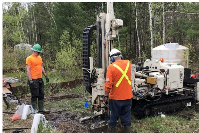
Photo: Technicians collect core samples from a hydrocarbon-contaminated aquifer near Barrie, Ont. U of T's Elizabeth Edwards and her partners have developed bacterial cultures designed to clean up such sites by breaking down contaminants (photo by Courtney Toth)
