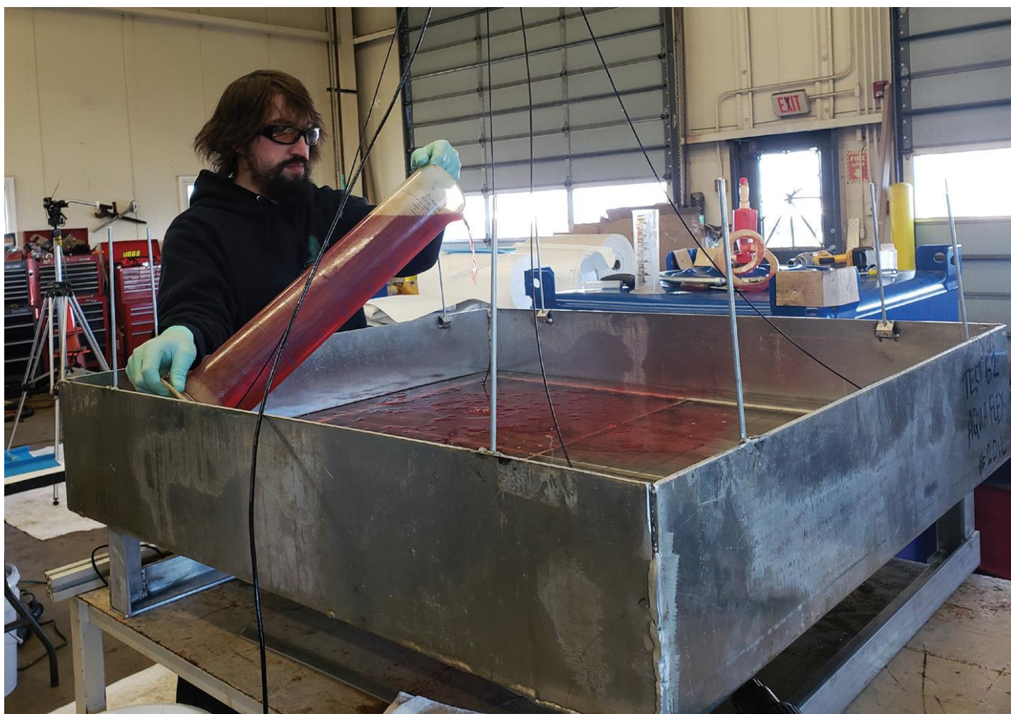
Ohmsett Technician Allen Cannone prepares the support rack with a known quantity of oil where sorbent samples would be placed. Sorbents were
