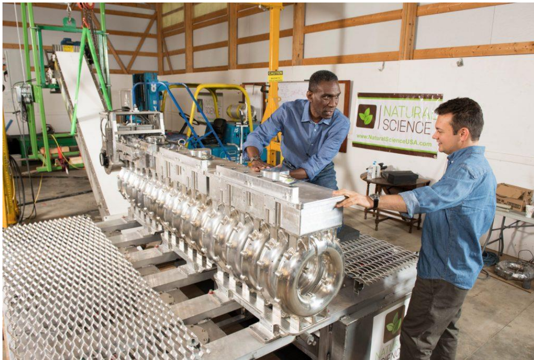
Photo: Scientist Arden Warner, left, shows Aaron Sauers, Fermilab licensing and patent executive, the E-MOP system. It consists of solenoidal (doughnut shaped) magnets that are coupled together in groups of six to form a module. Several modules are connected together to form an electromagnetic-boom (e-boom) structure. The system can be made longer or shorter by adding or removing modules to accommodate the situation. Every magnet in the structure is separated from the next by a fixed distance that optimizes the “gradient” effect of the magnetic fields between them. Photo: Reidar Hahn, Fermilab
