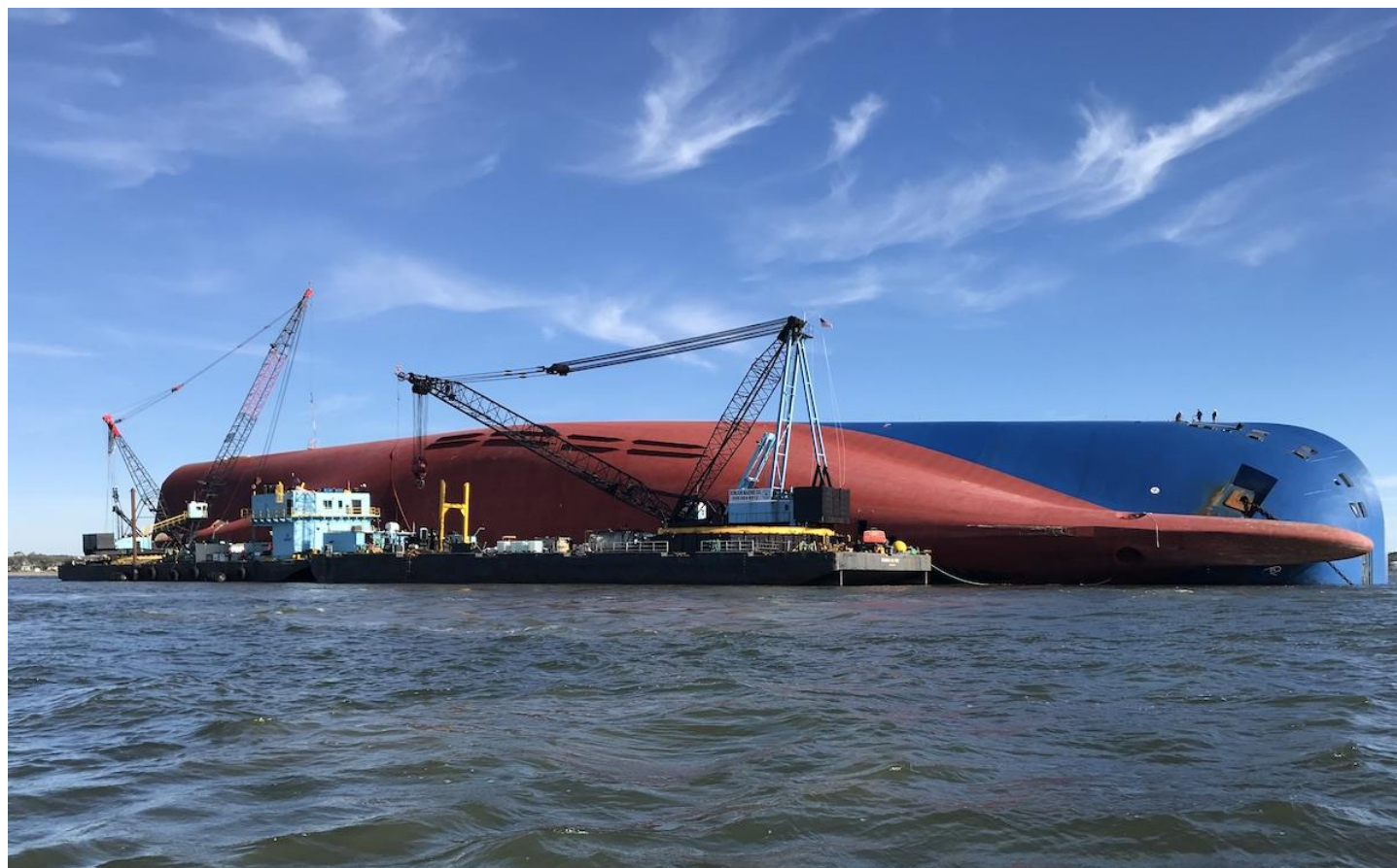
Photo: Crews onboard work barges work to clean residual fuel oil from tanks inside the M/V Golden Ray, St. Simons Sound, Dec. 3, 2019. Photo: St. Simons Sound Unified Command
