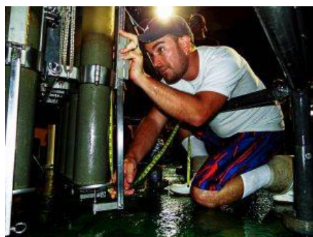
Photo: Patrick Schwing measures a sediment core from the sea floor. Courtesy of Devin Firesinger
