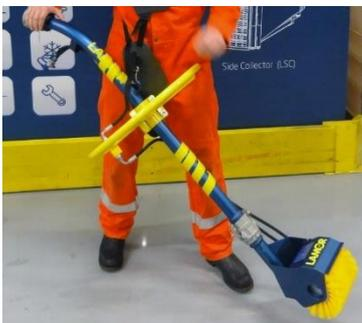
The LRC Rock Cleaner has a small hydraulic brush that removes oil from rocks and separates oil and water. The collected oil passes into the funnel behind the brush, from where the oil is sucked with a separate suction pump. The LRC Rock cleaner is controlled by a control handle and carrying harnesses.
