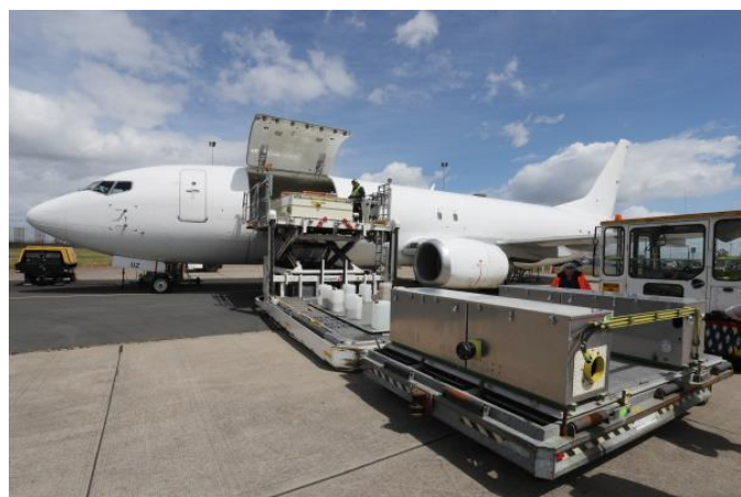
Photo: Boeing 737 using normal cargo loading converting it to an oil spray dispersion aircraft
