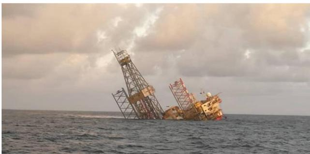
The Velesto Naga 7 was operating at the Salam-3 well for customer ConocoPhillips at the time of the accident. Velesto said the incident occurred due to rapid soil penetration, which caused the rig to list and subsequently sink. The company said the rig is now fully submerged at the location.
