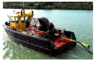
October 27 - Reel end, single point inflation, coastal waters lightweight system - Building on our patented technology, Super HI Sprint has undergone further development and in response to a customer requirement is now available in a smaller lightweight robust version making it ideally suited to small boats and protected waters (ports, harbours, terminals and coastal waters), ASTM F1523.
