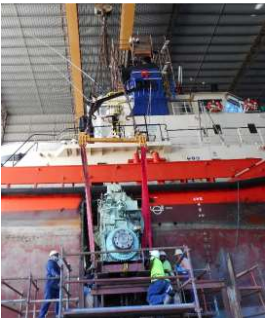
Left: Installation of the Waiowa’s new 19.7 tonne engine was performed by PacTow’s in-house workshop, maintenance, and engineering teams. Above: Pacific Towing’s ASD tug ‘Waiowa’ assisting Singapore flagged oil tanker ‘Crescent River’ in Port Moresby.
