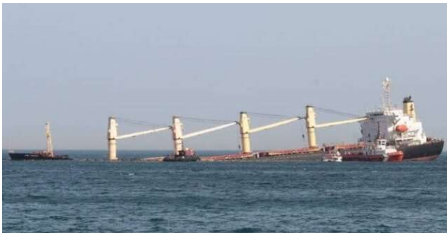
Above: The bend and break is visible near the number 2 hold of the OS 35. Photo Courtesy of Gibraltar Port Authority
