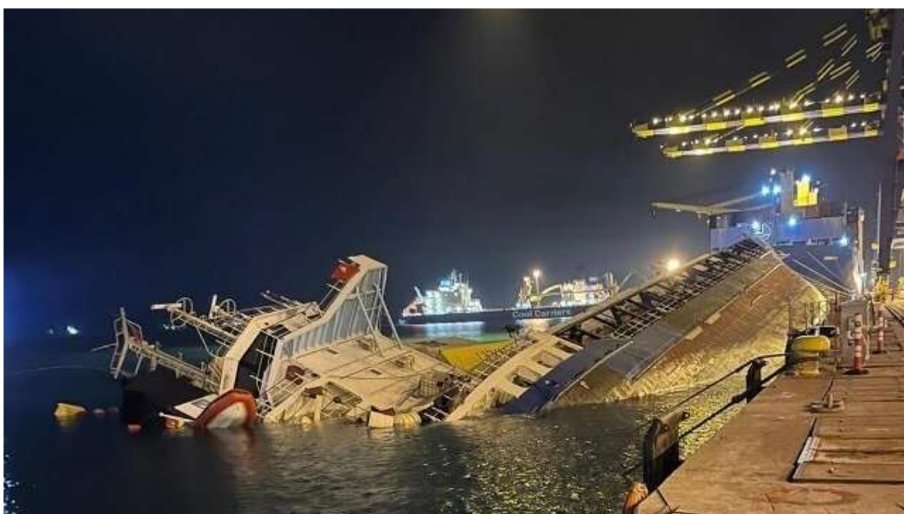
Sea Eagle resting on her side after losing stability (Photo courtesy of Turkish Ministry of Transport)
