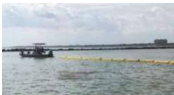
Biodegradable peat moss “mock-spill” being collected by the U-boom configuration
