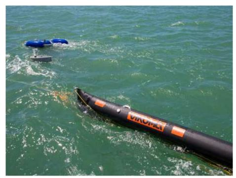
The Vikoma paravane is a powerful and versatile tool. In a traditional open water boom deployment it replaces the tow boat, enabling a single vessel to deploy a boom system.
