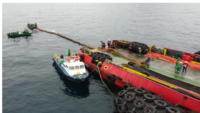
Deployment of Containment Booms
