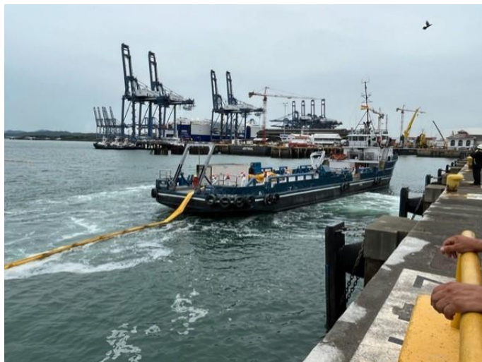
Deployment booms OSRV (Layne) – Port of Balboa
