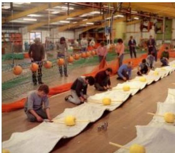
Pictured left: Boom assembly in progress at Jackson Trawl's Peterhead factory.
