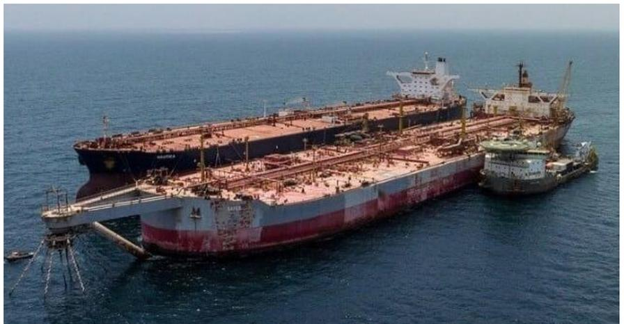
Above: FSO Safer oil transfer Crude oil tanker renamed Yemen is now alongside the FSO Safer as well as the Boskalis salvage vessel conducting the operation (Photo courtesy of Boskalis)
