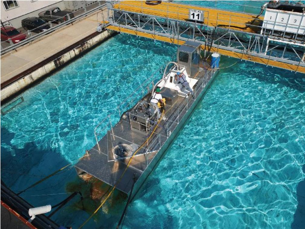
*Extreme Spill Technologies designed a new type of oil spill response technology that uses a vessel equipped with a pump system that takes advantage of the oil and water densities to separate the fluids.*
