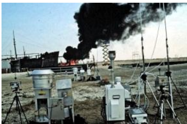
Figure 4 A test of fire boom in the early 1990's. All the instruments in the foreground are to measure or capture emissions.
