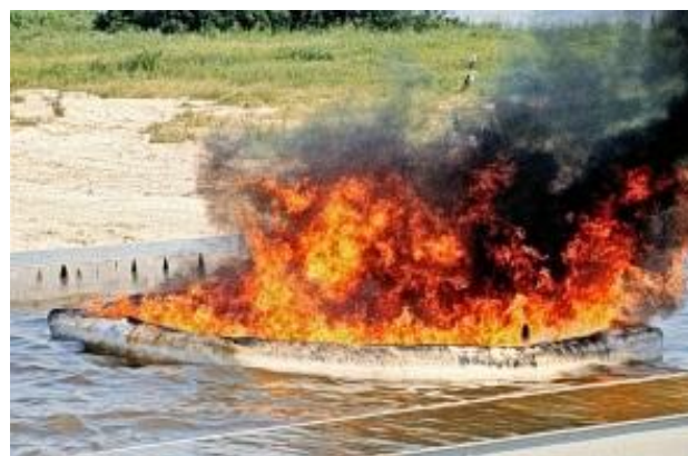
Figure 5 A test of fire boom at the USCG Mobile facility using the ASTM protocol. The emissions from this test would be been measured in a similar manner to that shown in Figure 4.
