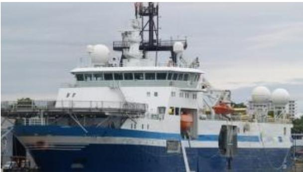
An OSRV is designed to respond to a discharge of oil and recover the oil dispersed on the sea surface
