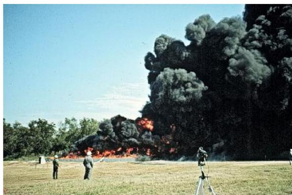
**Figure 14 (left)** A photograph of a mid-size diesel fuel fire in which the plume does not rise due to a inversion. Such cases are rare but result in worst-case situations for emissions.
