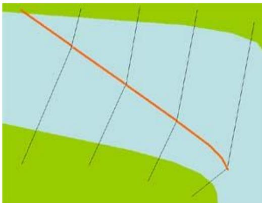
Booms should be anchored either in the river or on the banks to maintain the angle as good as possible. In currents of more than 1mps, shorter lengths of boom should be used to provide more anchor points at the connections.
