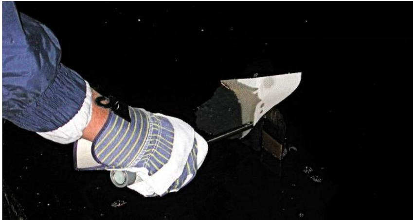
**Figure 18** The ignition of a heavy oil. This is easily carried out by adding a small amount of primer such as diesel fuel (about 20 mL), and adding a small wick such as cardboard or paper towel
