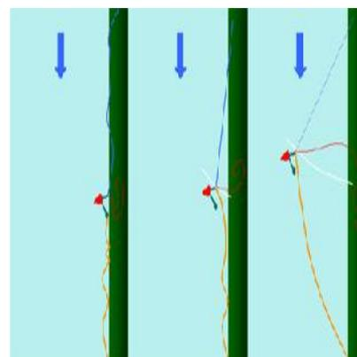
The system can be operated in rivers with heavy traffic as the Boom Vane control rudder allows for speedy and effortless retrieval from midstream.
