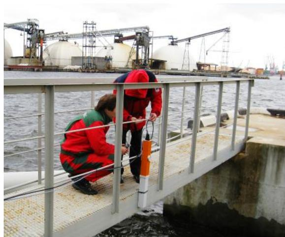
To detect oil slicks as thin as a single micron from up to 10m above the water, ROW pulses a UV beam at the surface and excites any oil molecules in the target area. Using oil's native fluorescence, ROW picks up the signal from tell-tale substances and alerts the site operator.
