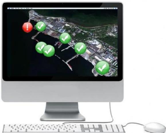
It is an early warning system that alerts you of oil leaks and spills, ensuring that small spills do not get out of hand. Industry leading sensitivity allows ROW to reliably detect surface slicks down to 1 micron. Using ROW's configuration software, alarm levels can be set to suit the client's needs and local environmental standards, minimising false alarms. Hermetically sealed and IP68 certified, ROW is designed to run autonomously in the toughest of environments.
