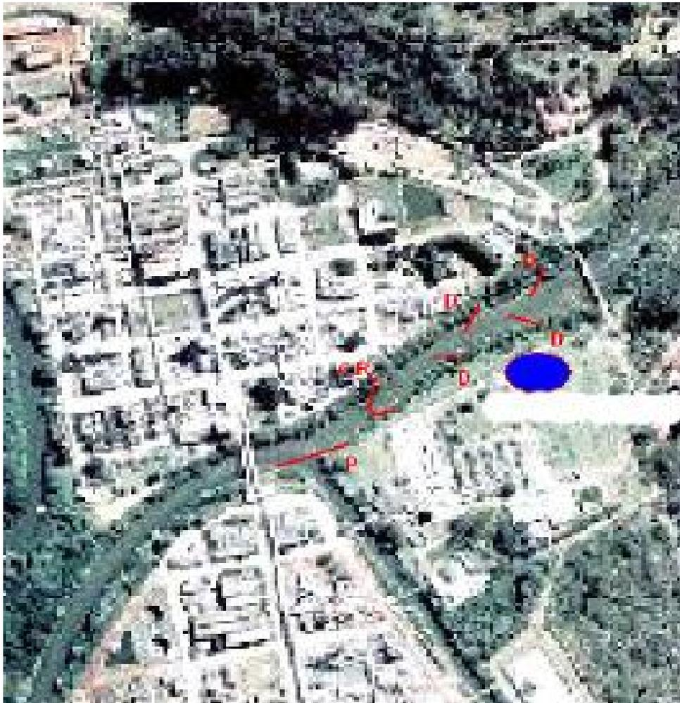
As can be seen the red lines (D) deflect oil into a (CR) U configuration where the apex is in the middle of the river, so recovery will be difficult. In fact oil will be lost.
