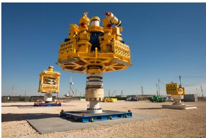
As demands by offshore operators have evolved, MWCC has had to evolve their technology as well. Last month they unveiled their newly up-rated capping stack with the ability to handle upwards of 350 degree fluid temperatures.
