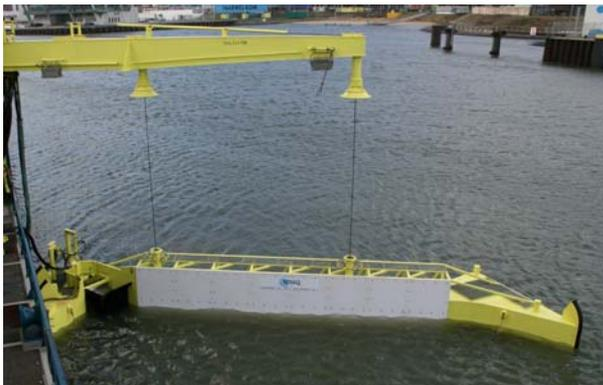
Koseq has tested a newly developed brush conveyor skimmer cassette in one of the rigid sweeping arms of the Rijkswaterstaat vessel Arca.
