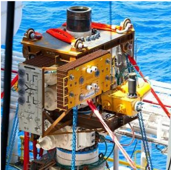
*Capping stack to stop flow and divert to vessels. This capping stack has been under construction for approx 2 months at the Cameron facility in Berwick, LA.*
