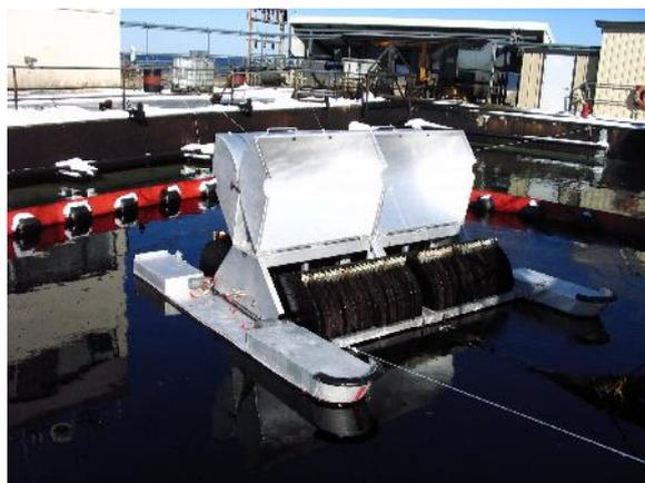
*In the picture: C-disc skimmer during testing at OHMSETT*
