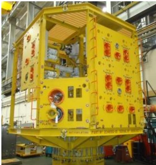
Your editor was able to view this major piece of new equipment, designed to be a key element of the UK offshore oil and gas industry's oil spill response capability. It has been constructed, tested and is available for deployment. The capping device was revealed on Tuesday 6th September 2011 by UK Energy Minister, Charles Hendry MP, at the SPE Offshore Europe 2011 conference in Aberdeen.
