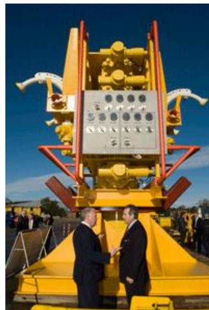
capping stack. For debris clearing activities, 660 and 2500 series shears are included in the package.
