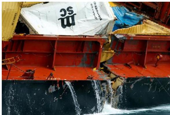
*A close-up view of the crack in the Rena's hull.
