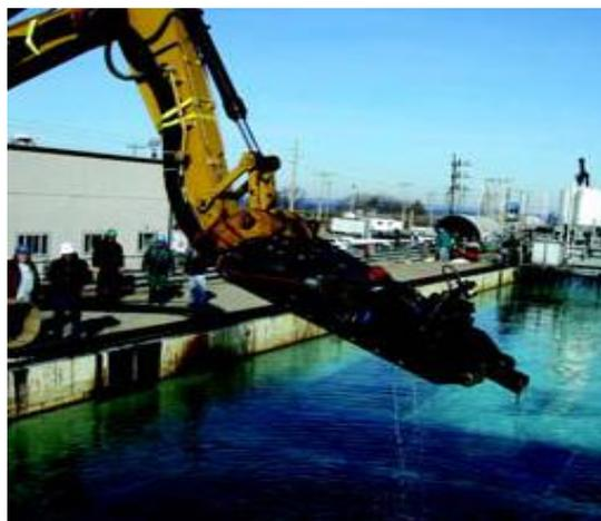
*Pictured left: Oil Stop's remote-controlled Sub-Dredge equipped with an EDDY pump, volute, and rotor, can go under, over, or around obstacles to remove sediment or oil*
