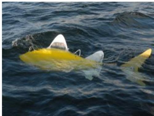
*The robots are battery powered and can run for 8 hours between charges (Image: Luke Speller)*
