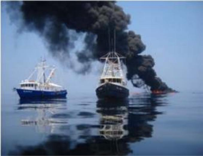
Picture on left - Fishing vessels towing fire boom – Gulf of Mexico 2010
