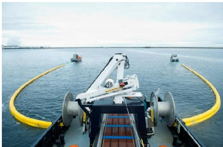
*Photo: The vessel Burrard Cleaner No. 9 demonstrates how its booms surround oil spills so they can be cleaned up.*
