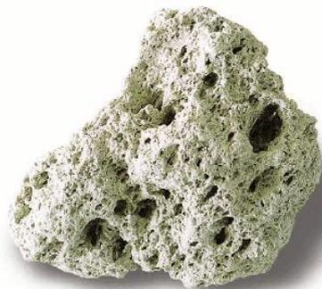
A new patented oil collection method is based on pumice stones from Icelandic volcanic eruptions which occurred thousands of years ago through a very thick ice glacier where the rapid cooling of the Pumice stone (approx. 3.5 cm in diameter) created small air pockets in the stones which made the stone very strong and light plus sufficiently waterproof to keep afloat for up to 5 weeks before sinking. The Pumice is sufficiently resistant to be cleaned and reused within a time span of 3-5 weeks.
