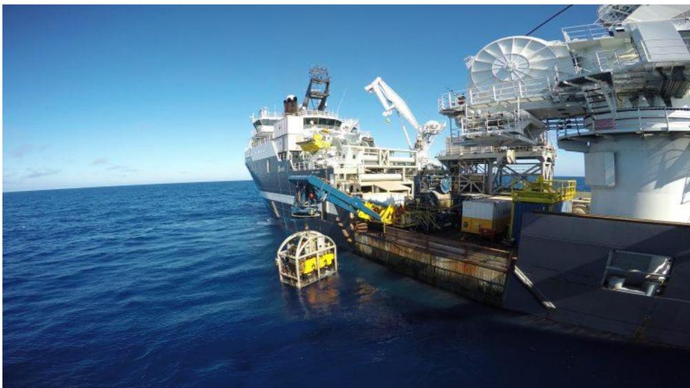
Photo: CANARY ISLANDS, Spain – In August 2015, Ardent and Ardentia performed a deep sea oil removal by means of deploying subsea recovery domes and oil receiving tanks operated by remote operated vehicles (ROV) from a diving support vessel. (Courtesy Photo)
