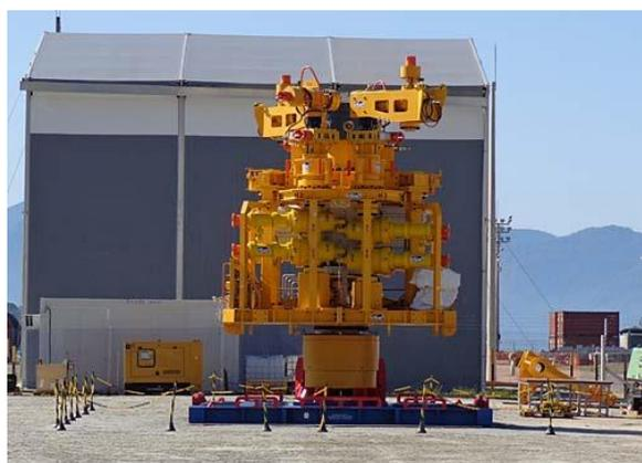
Photo: The 15k PSI Capping Stack at OSRL's base in Angra dos Reis, Brazil (photo: OSRL)
