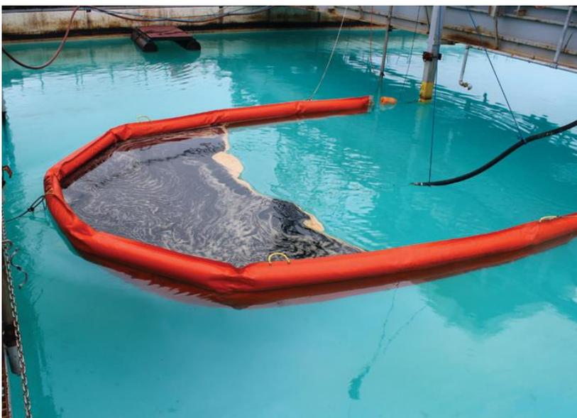
*Photo: During the diminishing slick thickness test, the skimmer recovery rate and efficiency was quantified using the ASTM F2709 guidelines while recovering from 3 to 2 inches of oil. Performance tests in thinner slicks included thicknesses of 2, 1, ½ and ¼ inches.*
